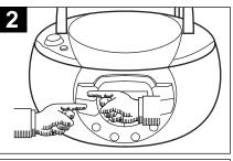
During playback, press the Skip/Search REV. (I◄◄) button once to move the player back to the beginning of the current track. Press the Skip/Search REV. (I◄◄) button repeatedly to move the player back to lower-numbered tracks.
